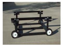
This picture shows the completed carrier without the tire in place. Note the bars on the top; they clamp to the frame rails in front of thru rear end and hold the removable carrier. The carrier is held to the mounting bars by 4 bolts with elastic stop nuts. The wheels allow the carrier to roll into place where the whole thing is winched up to its carry position by a 110 volt winch that can be purchased from Harbor Freight
