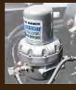
Chassis built before 11/28/03 have a Pure Air dryer, which is equipped with a spin-on desiccant cartridge that we recommend be changed every 18 months. Inside the air dryer is a coalescing filter that should also be changed every 18 months. Chassis built on or after 11/28/03 have a PURest Dryer with a scheduled change interval of 36 months.
